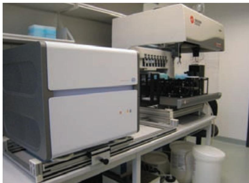
**Figure 16:** Example of a BeckmanCoulter Biomek® NX qPCR workstation integrated with Roche LightCycler® 480. The LightCycler® is mounted on a sliding tray to provide for easy disconnection of Biomek® and LightCycler®. The LightCycler® can be accessed manually during the run of a Biomek® pipetting method or can be controlled from within the Biomek® software for complete automation of qPCR
