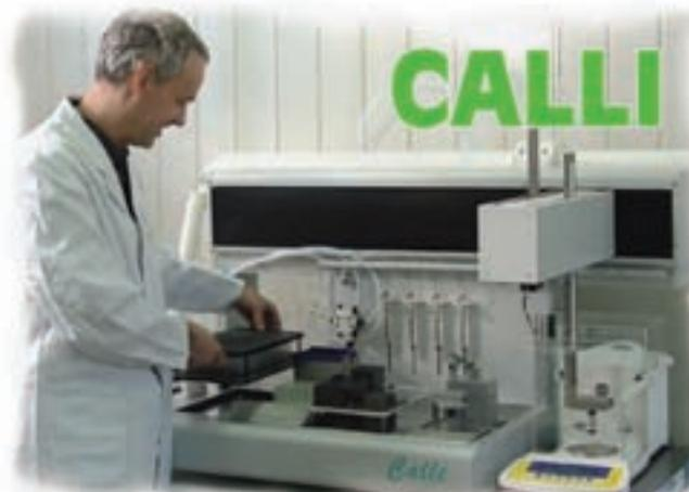
**Calli® LH** weighing and liquid handling system calculates dilution volumes, reads barcodes, and prepares screening plates. The optional **Calli®-plus software** offers useful sorting functions for "Cherry picking" of vials and micro tubes by individual sample properties and database entries.
