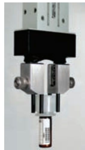
Figure 13 Mettler-Toledo's FlexiWeigh workstation for many-to many dispenses (left) with close-up of robotic gripper holding a FlexCap dispensing head fitted to a bar-coded source vial (right)
