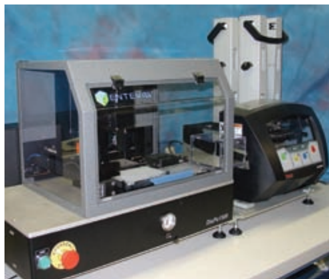
Figure 10: The BioDot DisPo™ 1500 Powder Dispensing System with Plate Stacker. The automated platform includes programmable mass ranges, absolute mass record via an integrated 5 decimal place balance, plate shaking/vibration of powder samples, electrostatic control with chamber ionisation, and on board wash station for sample probe cleaning (to minimise carryover)
