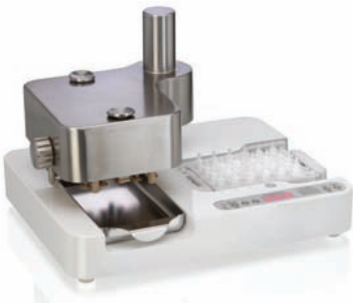
Figure 24: The RAFT (Real Architecture for 3D Tissue) system from The Automation Partnership forms tissues in less than an hour by controlling compression and incubation of collagen-based gels seeded with cells. The system, which uses a SBS standard 24-well plate format can be filled manually and will fit into a standard laminar flow hood to prevent contamination of tissue constructs
