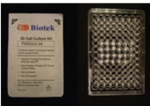
Figure 8: 3D Biotek 3D Cell Culture Kit which contains 24 96-well 3D Insert™-PS scaffolds
