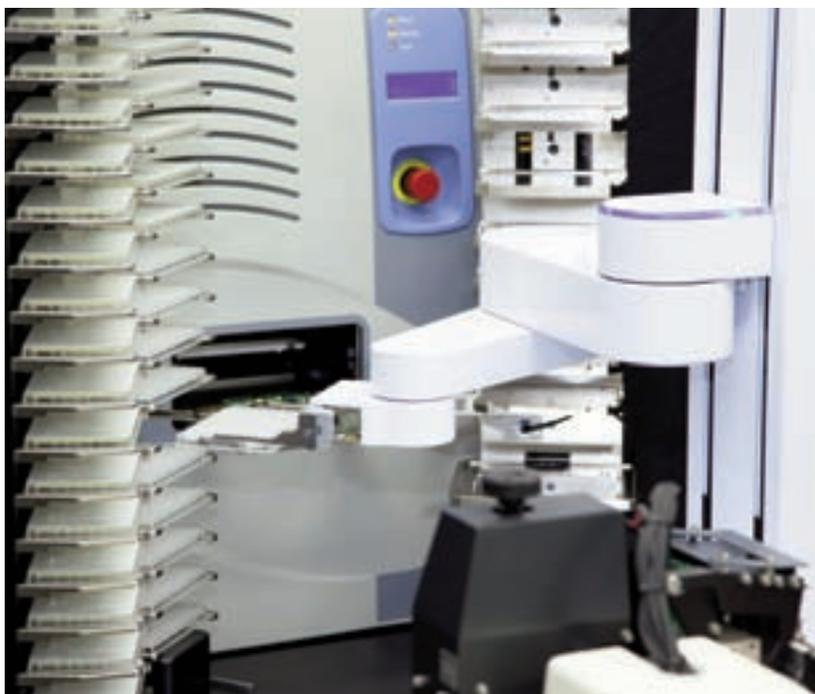
**Figure 19:** The Access™ laboratory workstation from Labcyte supports the wider application of Echo liquid handlers
