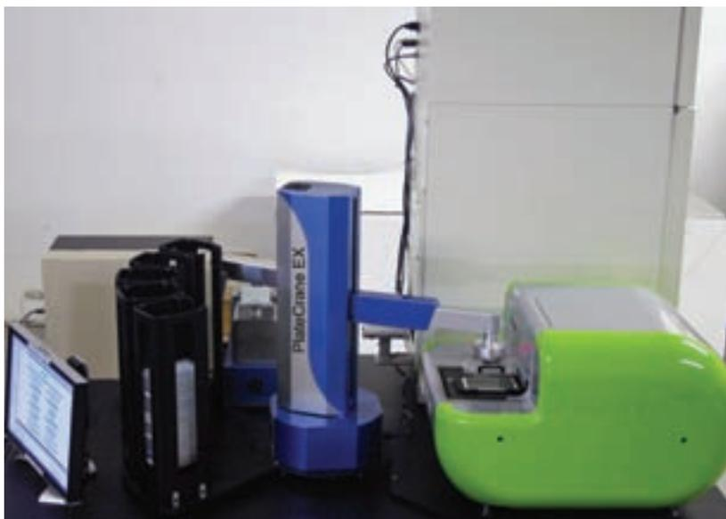
**Figure 18:** Front left: Hudson PlateCrane EX with 5 stacks, Hudson PA1000 Barcode Print & Apply in back left, Liconic STX110 incubator in back right and Genetix CloneSelect Imager in front left. System will apply barcodes to plates either on the fly or as an off-line process. Plates are loaded into the incubator, then removed on schedule to the reader, then back to incubator. Data is collected and logged. User is alerted by email to any errors, exceptions and the end of the process
