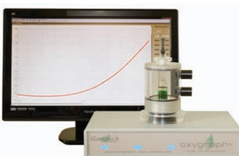
**Figure 14:** The Hanstech Instruments Oxygraph Plus oxygen electrode system
