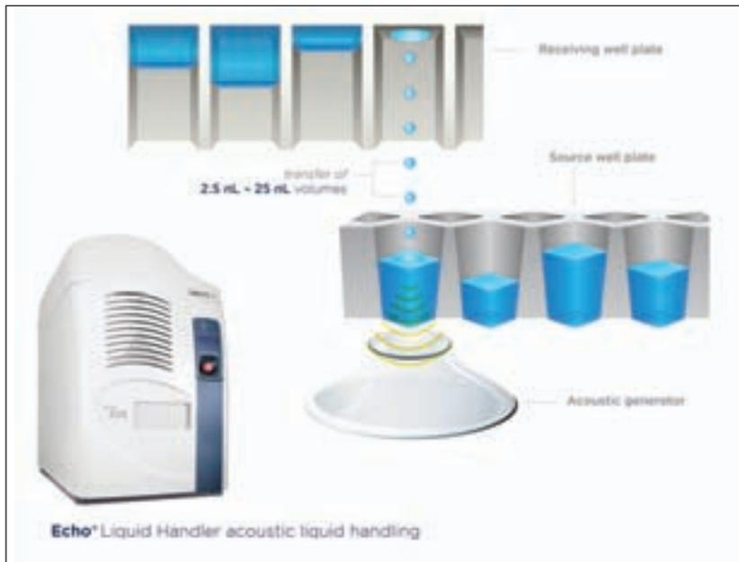
**Figure 18:** Diagram of acoustic liquid transfer process. Labcyte Echo 525 liquid handlers transfer 25 nanolitre droplets of samples and assay reagents from microplate wells using only acoustic energy. Droplets are rapidly transferred to build larger volumes in seconds. Transfer without the use of tips, capillaries or similar devices eliminates sample carryover to assure great accuracy and precision across its transfer volume range (25nL to 10µL)
