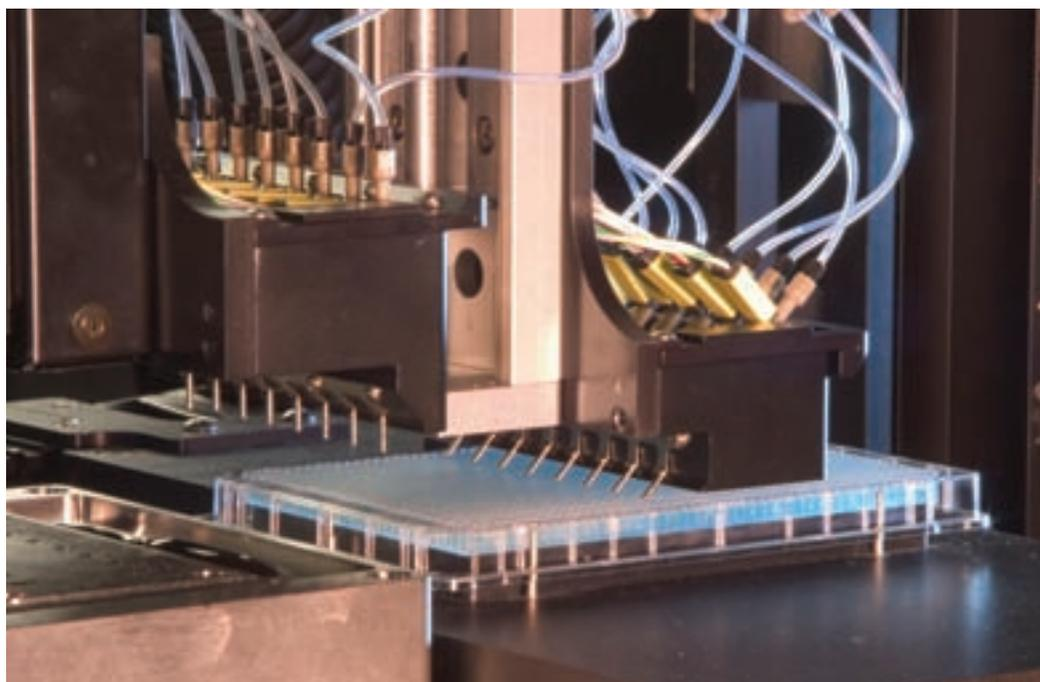
**Figure 18:** 384/1536 DA unit with clog detection and recovery from Wako Automation, powered by Kalypsys Systems
