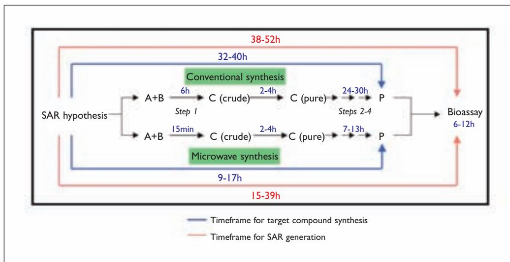
**Figure 1:** SAR Cycle, comparing conventional and microwave synthesis
