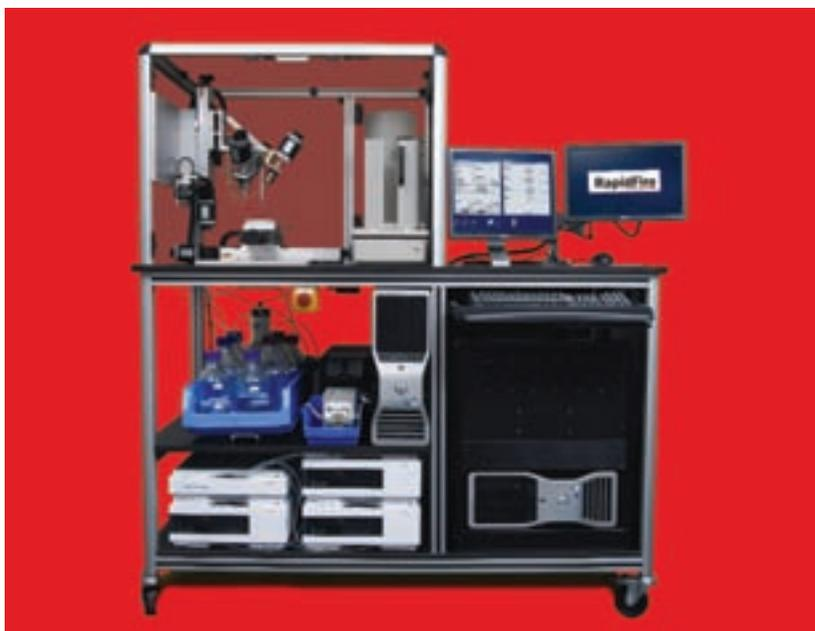
**Figure 12:** The Biocius RapidFire® RF300 Mass Spectrometry System processes epigenetic samples in 6-8 seconds each
