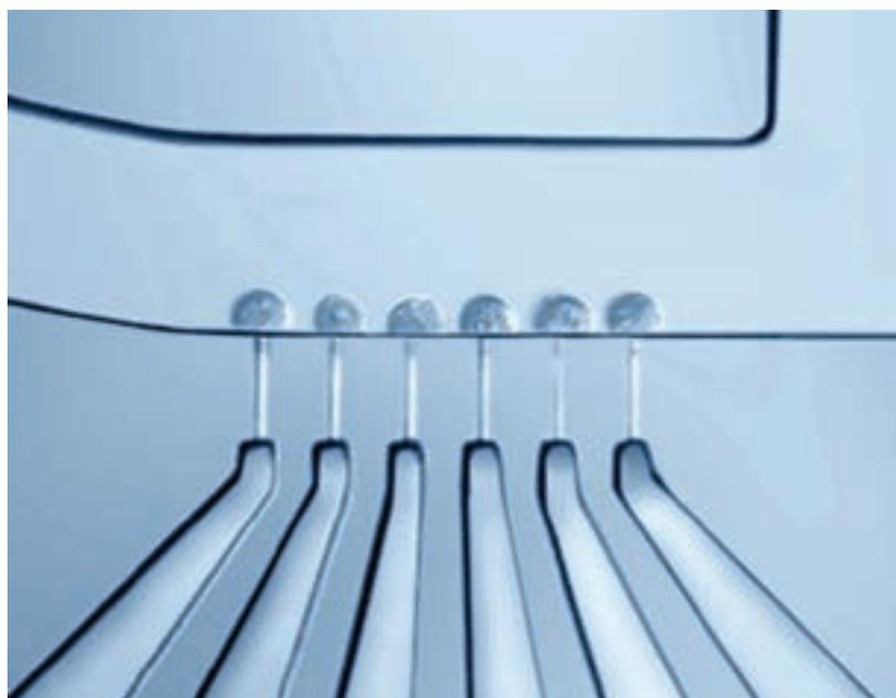
**Figure 14:** Image showing a cell trapping zone in the microfluidic patch clamp plate utilised in Celectricon's Dynaflow®HT system
