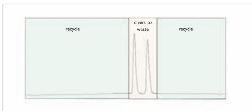
**Figure 2:** Solvent savings by recycle of 'clean' eluent. A switching valve can be used to recycle effluent from regions of the chromatogram containing no peaks (green areas – about 85% of total solvent)
