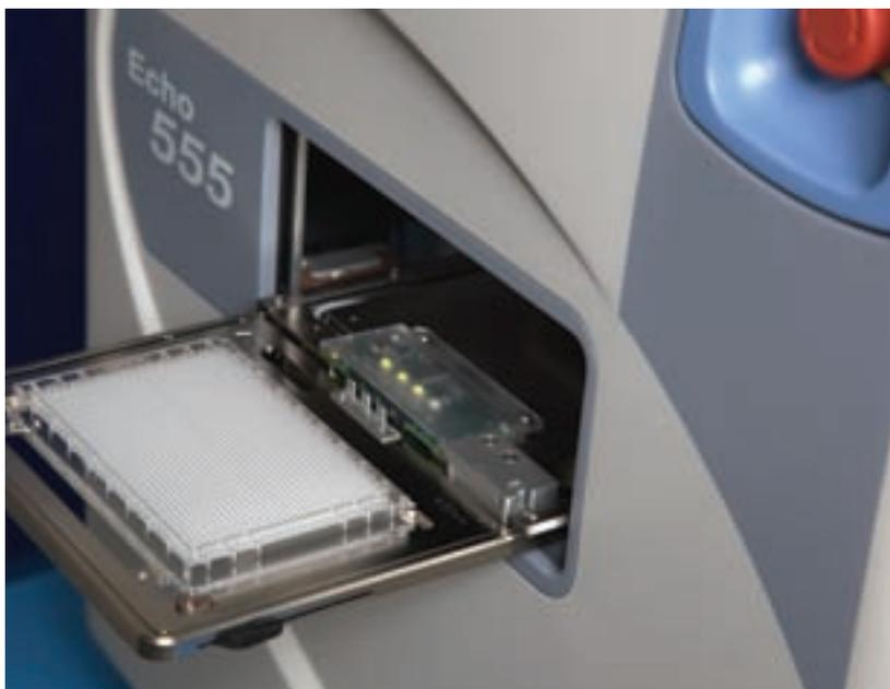
**Figure 18:** An acoustically engineered, 1536-well, Echo qualified source plate on the source plate stage of an Labcyte Echo 555 acoustic liquid handler
