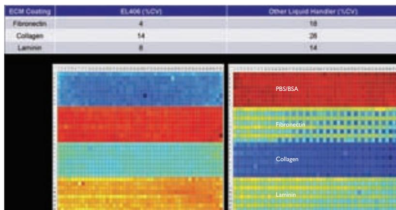
**Figure 11:** Cell-based assays based on label-free detection with SRU's BIND® platform were prepared in 1536-well microplates using the BioTek EL406™ for the sequential dispensing of microplate coatings (fibronectin, collagen or laminin) and cells expressing the target of interest. The figure shows a heat map comparison demonstrating the reproducibility of protein extracellular mix deposition across a 1536-well biosensor microplate for both the EL406™ and another liquid handling device
