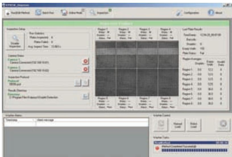
**Figure 17:** The software interface of Kalypsys Systems' new tip clog detection and recovery system on its 1536 Well Washer/Dispenser
