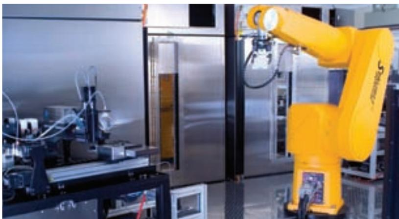
**Figure 16:** GNF Systems' compound profiling system; a 384/1536 well compatible high throughput screening system optimised for profiling libraries of compounds against tens to hundreds of cell based assays
