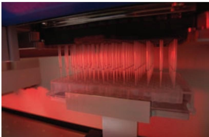
**Figure 21:** Precision replication of samples on 96-well plates prior to screening against enzyme panels using a PlateMate plus liquid handler at the International Centre for Kinase Profiling in Dundee
