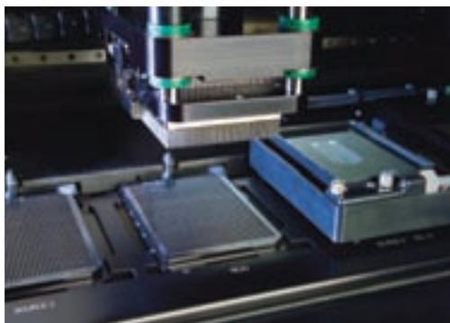
10nL to 50nL. Both pintool and pipette heads are interchangeable in the same protocol. Like the FDSS 6000, the FDSS 7000 has two modes of detection: fluorescence and flash luminescence. However, the FDSS 7000 now has a more sensitive luminescence sensor with better resolution. This is particularly important for Aequorin assays in 1536 well format because of low signal intensities. The improved sensitivity even allows for detection of most blue SPA (radiometric) assays (Figure 11).
