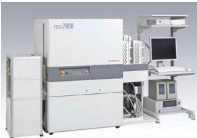
unique features that customers found useful in FDSS 6000, most noticeably the design of dual dispensers and integrated stackers. Dual dispensers isolate sticky agonists from compounds thus eliminating carryover artifacts. Further, the FDSS 7000 has three wash stations with a sonicator plus a tip
