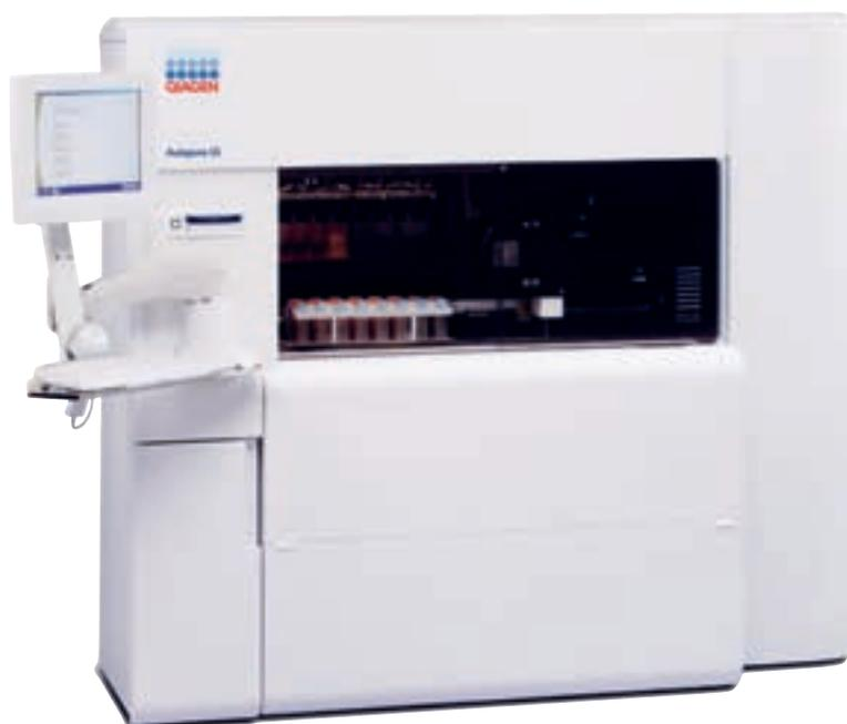
**Figure 17:** The Qiagen Autopure LS enables walk away purification of highly stable DNA ready for use or archiving
