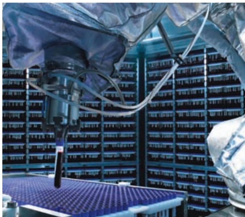
**Figure 10:** From inside deCODE Genetics Sample Vault industrial robots can cherry-pick vials from storage trays and verify by barcode. Here shown picking 9mL vacutainers
