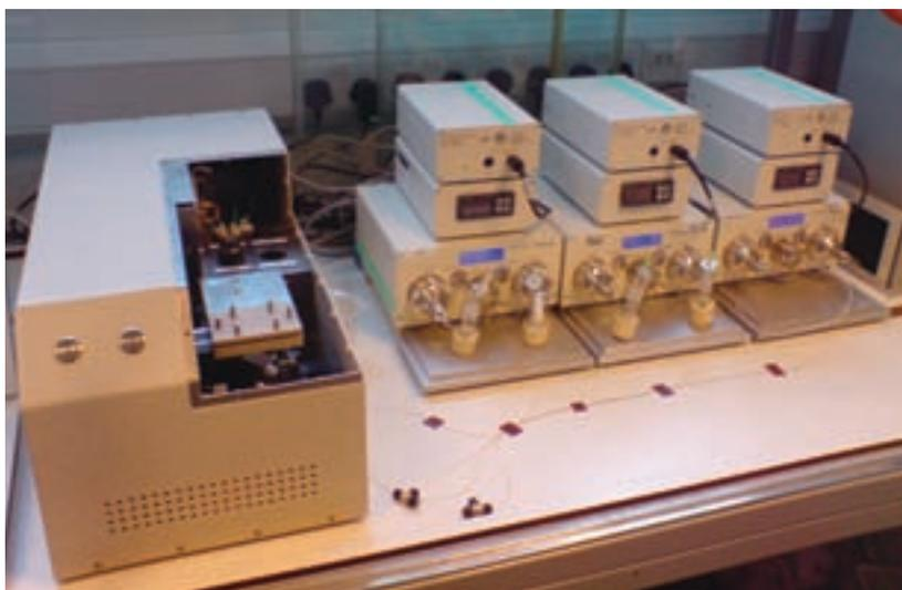
**Figure 13:** Genapta's direct dilution IC<sub>50</sub> engine. Compounds are introduced as single samples in the milli-molar regime. They are diluted and assayed automatically by the system without the intervention of any external sample handling or automation. The device is capable of producing a 100-200 point IC<sub>50</sub> curve in 30 minutes using just a few microlitres of reagent. (Photo courtesy Ley Group, Dept of Chemistry, Univ of Cambridge)
