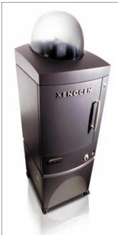
One of the newest products to market, the IVIS Spectrum, combines spectral unmixing capabilities with 3D tomography for both fluorescent and bioluminescent reporters. Available through Caliper Life Sciences. Image credit: Caliper Life Sciences
