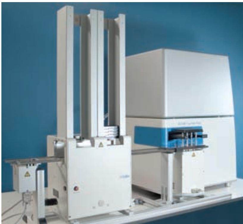
**Figure 11:** Small and powerful cellular screening workstation from CyBio: CyBi@-Lumax flash with one stacker and a comprehensive range of extension possibilities
