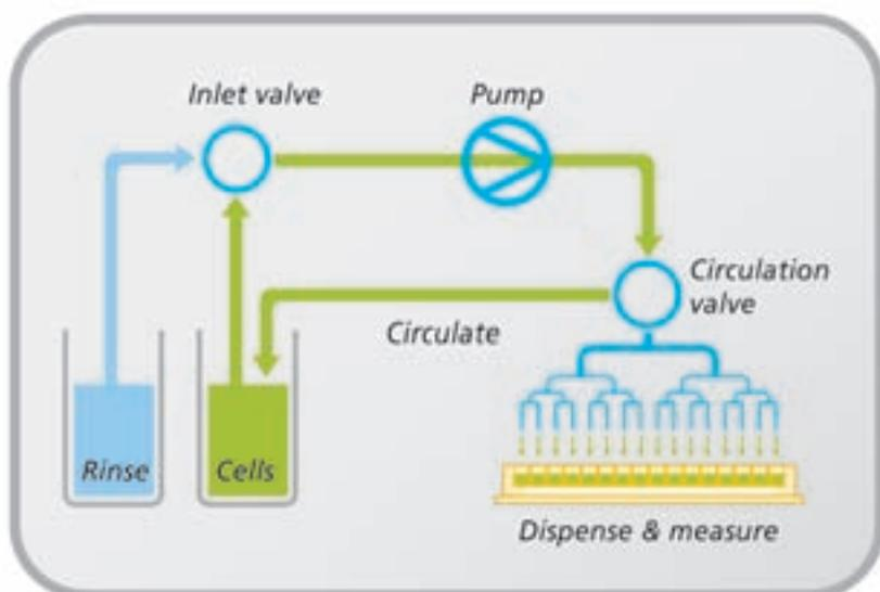
**Figure 10:** Schematic diagram of the cell circulation function and the patented multichannel droplet generator (EP 1 036 594) of the CyBi@-Lumax flash
