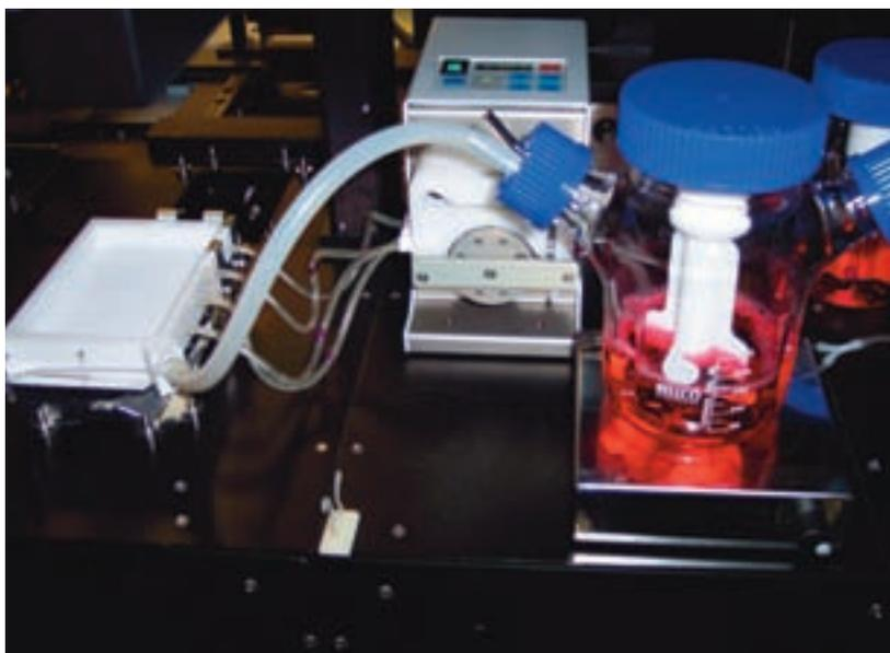
**Figure 20:** The new LumiLux cell stirrer mounted on a magnetic stirrer maintains cells in homogeneous suspension until ready for use. Cells sufficient for one microplate are pumped into the dispense tray and aspirated using the 384 tip dispense head. The remaining cells are returned to the cell stirrer flask or waste flask when the dispense tray tilts. 1000mL, 500mL, 250mL and 100mL cell stirrer flasks are now available for use in both assay development and screening
