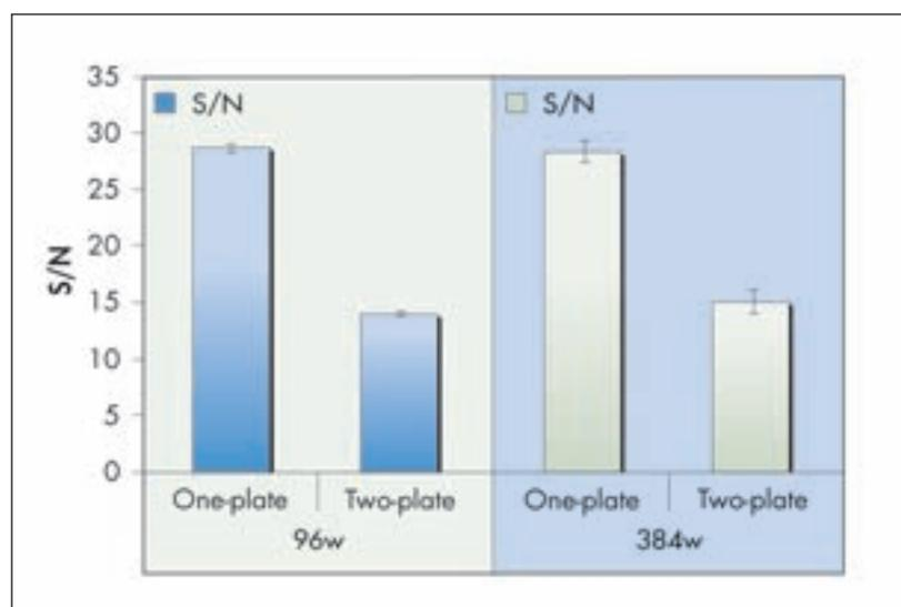
**Figure 4:** Comparison of signal to noise (S/N) in 96-well and 384-well MultiScreen glass-fibre filter plates using the two-plate vs one-plate methods (see Methods)
