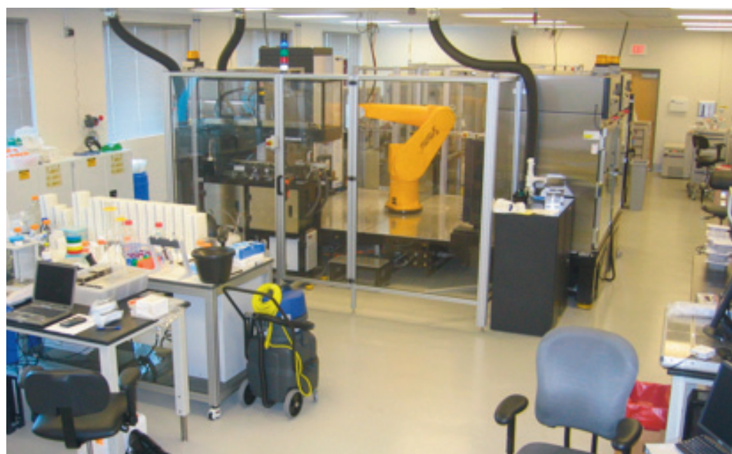
Figure 3 Scripps Florida's uHTS automation room. Assay development, compound management and uHTS operations are housed in a 1,800ft 2 class 10,000 clean room
