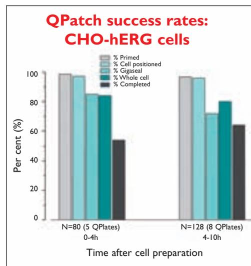
Sophion QPatch-16 workstation with on-board cell preparation device, showing the stirring apparatus (top left) and Q-fuge (on right, in front of the compound plate). Sophion QPatch success rates plotted as a function of the time after on-board cell preparation. Experiments were done with CHO cells expressing hERG potassium channels
