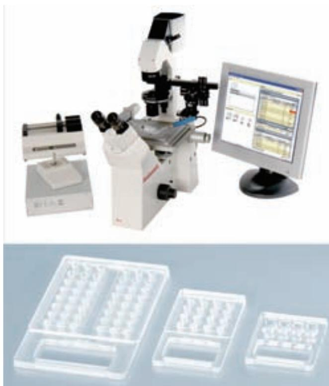
Collectricon Dynaflow Pro II System (top) is easily installed on an existing patch-clamp rig and consists of: Scan Stage, Pump, Commander Software, Controller and Microfluidic Chips (8-, 16- and 48-channels). A close-up (bottom) of a patch-clamped cell and the laminar flow zones at the channel outlets of the Dynaflow Microfluidic Chips
