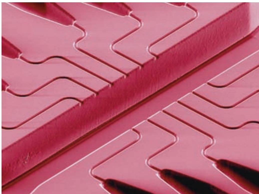
SEM of 12 channel patch clamp array chip developed by the BioPOETS group at UC Berkeley
