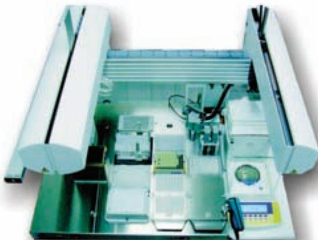
**CALLI** is a robotic calibrating, weighing and liquid handling system with a built in robotic arm. It reads barcodes on vials, micro tubes and plates, determines the tare weight, the weight of the contents and then calculates the volume of the solvent required for dissolution.
