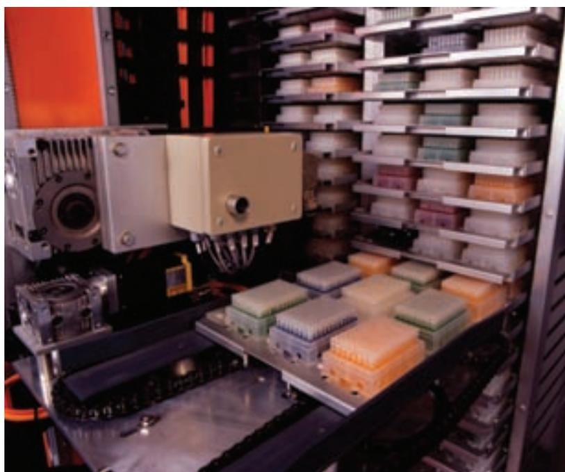
A typical RTS Life Sciences CompactStore™ which can hold up to 2,000 tubes per tray
