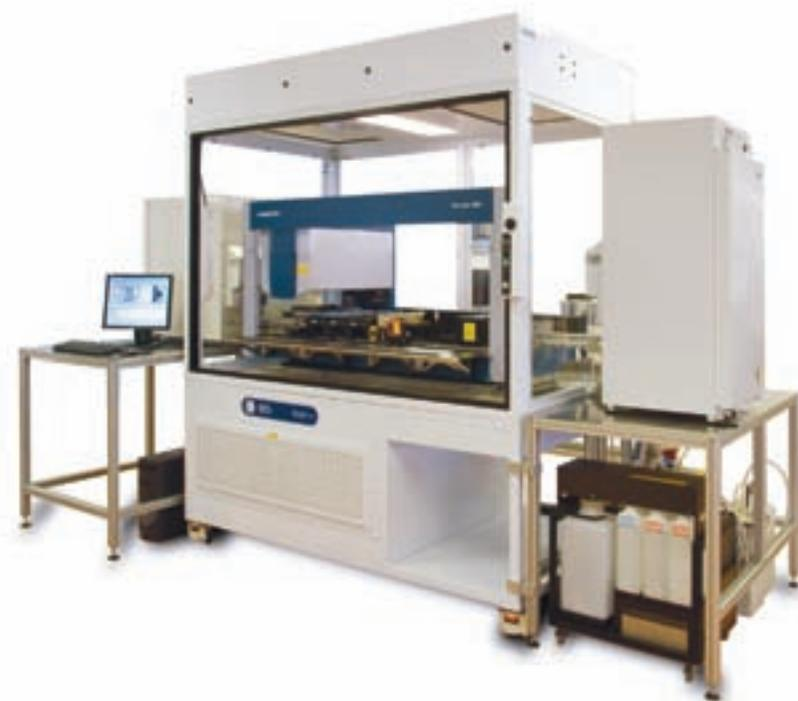
Hamilton Cell<sup>host</sup> System with 2 Kendro incubators (37°C incubator for cell cultures; 4°C incubator for media) and MICROLAB® STAR pipetting workstation contained in a sterile housing with laminar downflow
