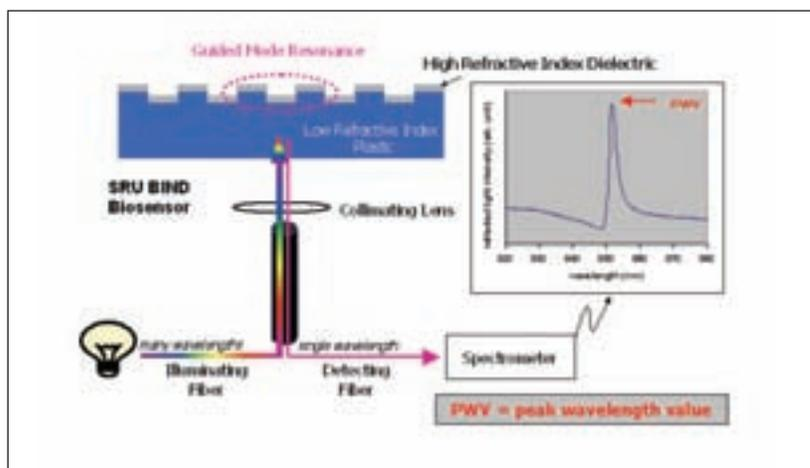
**SRU Figure 1 (above):** Schematic diagram illustrating the principle of operation of the SRU BIND™ sensor
