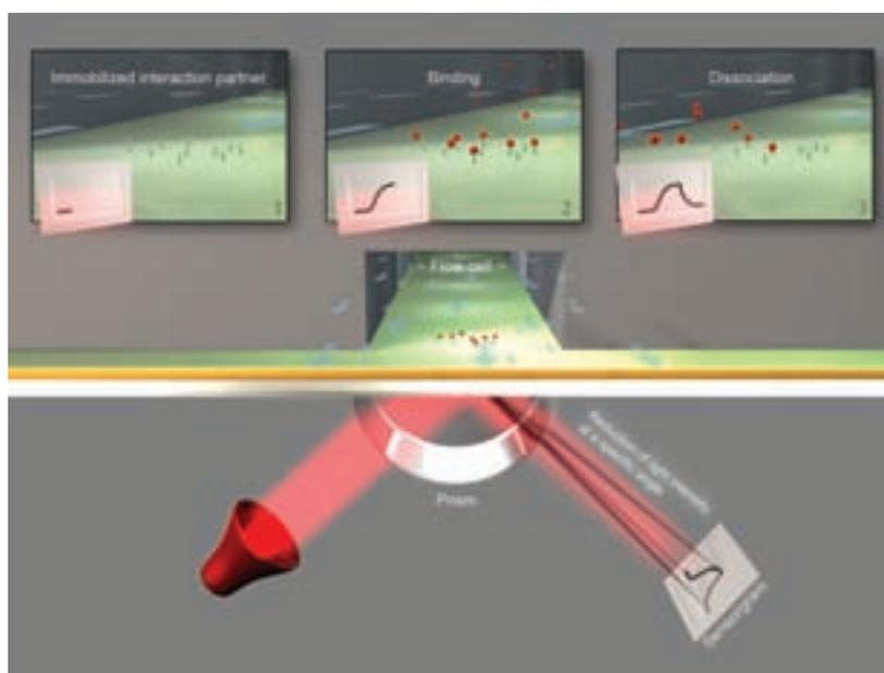
**Biacore Figure 1 :** Principle of surface plasmon resonance (SPR) on the Biacore. A flow cell is formed when a sensor surface encloses an open flow channel through which a solution containing analyte is injected. As the analyte passes over molecules immobilised on the sensor surface, the association and dissociation phases of the interaction are recorded in real time on a plot called a sensorgram
