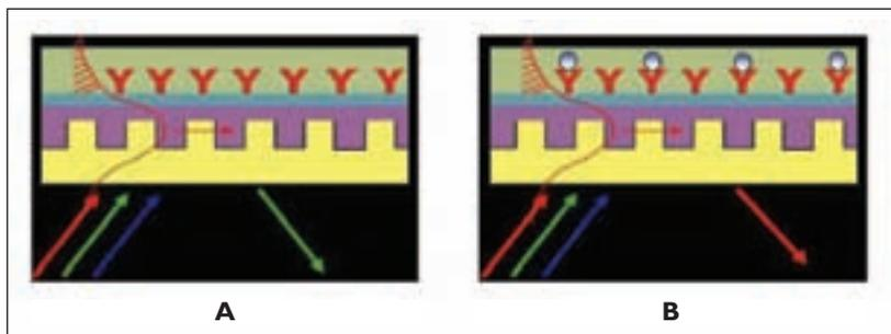
**Corning Figure 1:** Principle of Corning's Epic™ System. A) Biosensor without added analyte has given resonant wavelength; B) Binding analyte to target molecule gives resonant wavelength shift
