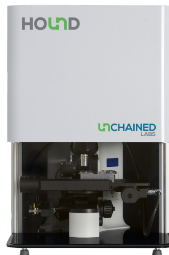
Figure 1: Hound images, sizes, counts and identifies particles with Raman or Laser-Induced Breakdown Spectroscopy.
