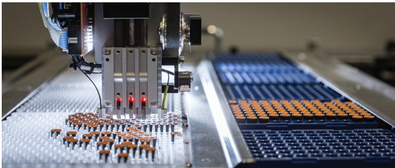
High-density storage trays holding sample tubes compatible with acoustic liquid handling
