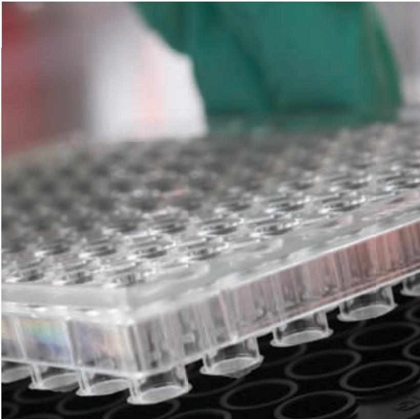
**Figure 16:** Corning's 96-well spheroid microplate and HTS Transwell®-96 tissue culture system
