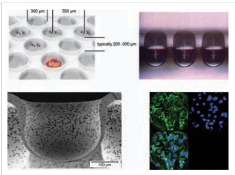
**Figure 13:** 300MICRONS microcavity arrays with principal design characteristics (upper left), light microscopic image (upper right), after the introduction of pores (lower left, scanning electron microscopy image) and appearance in high-throughput-/high-content-screening applications (lower right, confocal laser scanning microscopy image)
