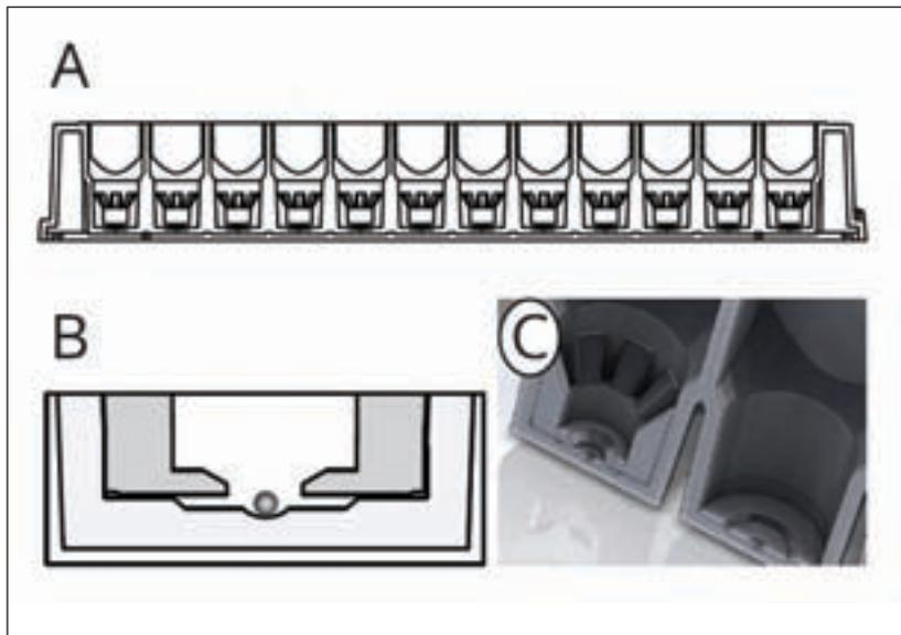
**Figure 14:** Schematic of an Agilent Technologies Seahorse XFe96 Spheroid Microplate showing: 1) unique geometry; 2) the correct position of the spheroid at the bottom of the well. The plate is designed to hold spheroids between 200 and 500µM in diameter; and 3) the venting system that allows the optimal media mixing around each spheroid
