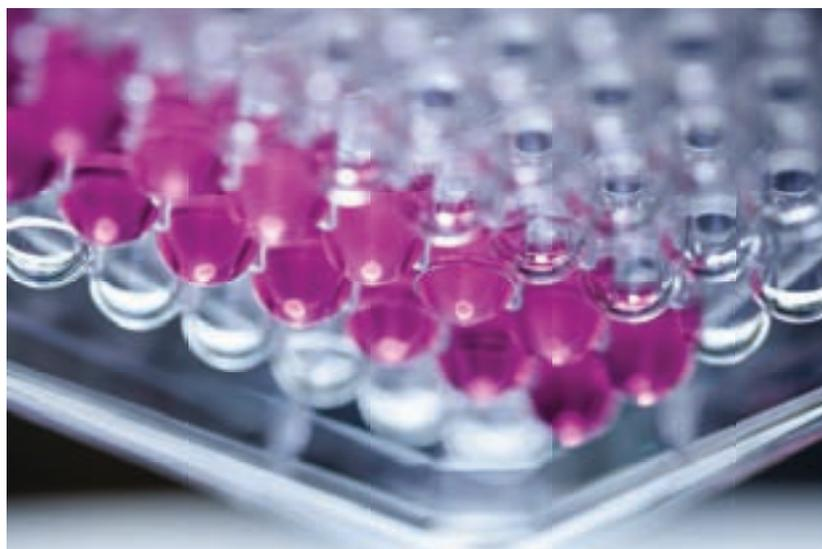
**Figure 17:** 96-well round bottom Greiner Bio-One CELLSTAR® microplate with cell-repellent surface to enhance the formation of a single spheroid per well
